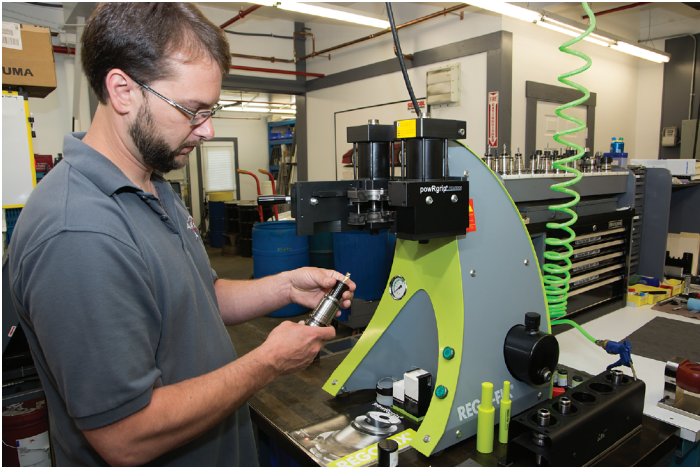
Tony Chastenay, All Axis R&D Owner and Operator. All Axis' REGO-FIX powRgrip push-button automatic unit loads/unloads tools in less than 10 seconds. The unit accommodates five different powRgrip collet sizes.
